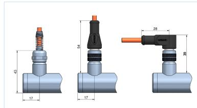
Sensors with cable output have a cable fitting and a spring for bend protection of the cable. The standard cable length is 2 m.
