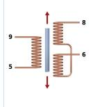
assignment for TPE-cable: primary 2 white (5): black (6): secondary 2 brown (9): primary 1 blue (8): secondary 1 assignment for PTFE-cable:
