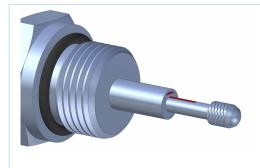
The option VH should to be chosen, if the sensor is used in liquids (oil, water, ...) or if fast pressure variations may occur. By milling plane surfaces on parts of the mechanics (see picture red marked) the pressure balance or venting of the inside area will be improved.
