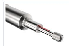
The option VH should to be chosen, if the sensor is used in liquids (oil, water, ...) or if fast pressure variations may occur. By milling plane surfaces on parts of the mechanics (see picture red marked) the pressure balance or venting of the inside area will be improved.
